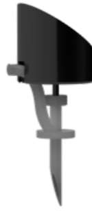
Figure 2.6: Needle assembly, consisting of the hard metal introducer needle surrounded by the flexible indwelling cannula. The metallic needle goes through a rubber stopper. A tube is connecting the indwelling cannula and the tank to enable drug flow.
